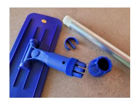
STEP 2 Unscrew the cap from the pad holder and remove the ring pin
